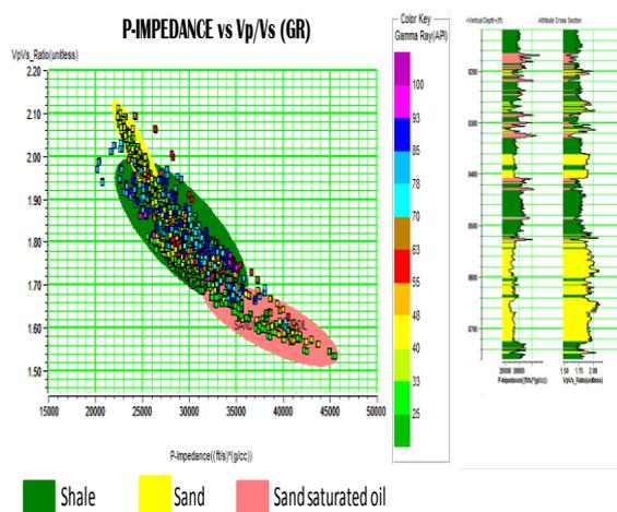
Figure 5. Cross plot of Vp/Vs ratio versus acoustic Impedance as function Gamma Ray using the estimated S-wave velocity from of #L-30, Penobscot field, Nova Scotia Basin, Canada.
