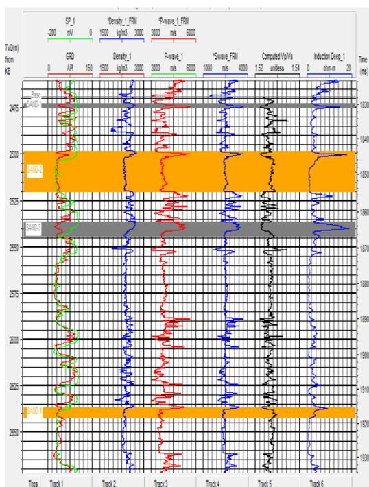
Gambar 4. Log data of #L-30 well containing oil saturated sandstone from Middle Missisauaga formation
