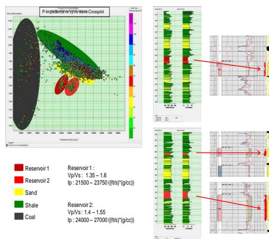
Figure 3. Cross plot of Vp/Vs ratio versus acoustic Impedance as function Gamma Ray using the estimated S-wave velocity from #PMK-2 well, Mawar field, Kutai Basin, Indonesia.
