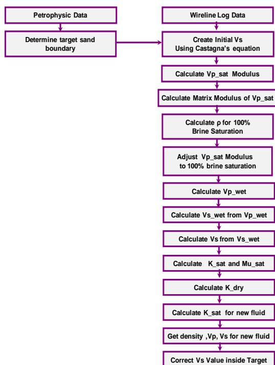
Figure 1. Workflow of S-wave velocity estimation using fluid replacement modeling
