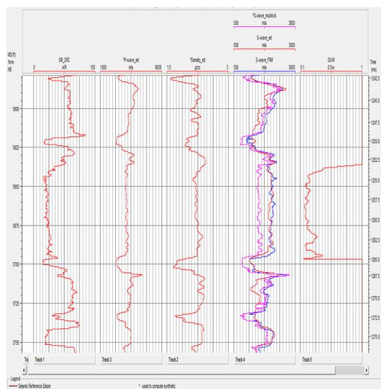
Figure 2. The comparison of original S-wave velocity, S-wave velocity estimated using fluid replacement modeling method and direct Castagna's relation from #PMK-2 well, Mawar field, Kutai Basin, Indonesia.
